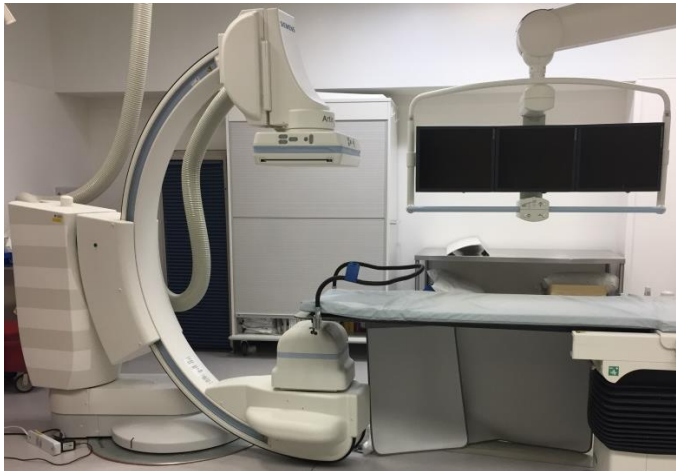
Figure 1-1. Example of a C-arm fluoroscope used for FGI procedures.
