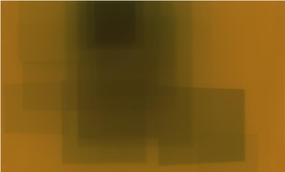
Figure 1-2. Radiochromic film (14 inches × 17 inches) from a fenestrated and branched endovascular repair showing the 2-dimensional radiation dose distribution. Film darkness correlates to increased radiation dose.
